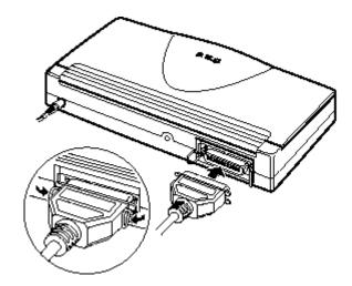
3. Connect the other end of the interface cable to the parallel interface port on your computer.
